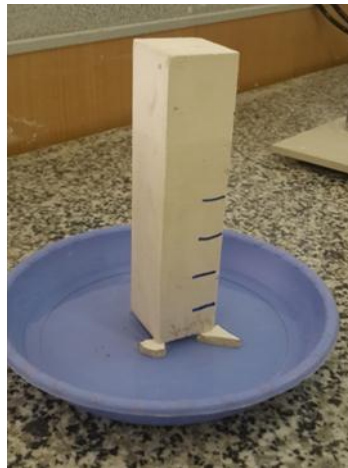
Fig.2. Measuring of water diffusion coefficient.
