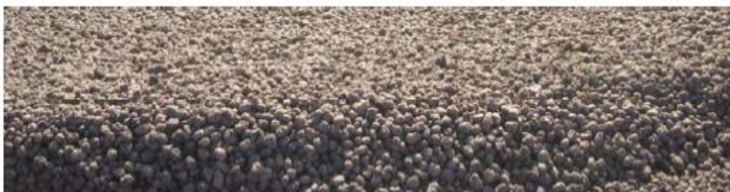
Fig.4. The close-up of placed LECA.
