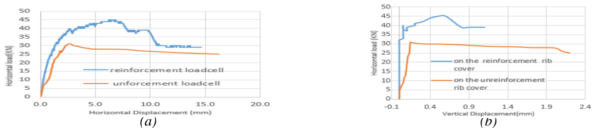
Figure 10. Comparison of the force-displacement diagram in reinforced and un reinforced structures: a) Horizontal displacement b) Vertical displacement.
