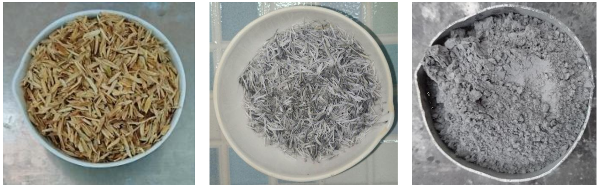
a. Rice husk ash (RHA) b. Burnt rice husk ash (RHA) b. Ground RHA used in making concrete
