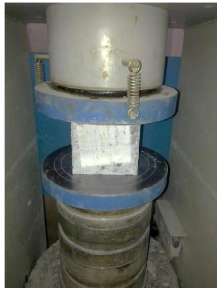
Figure 8. The cubic concrete sample under the compressive jack.
