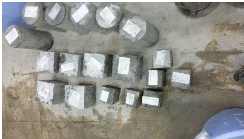
Figure 7. Air-dried concrete samples.
