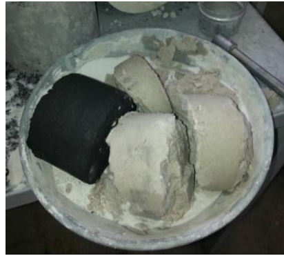
Figure 2. Difference between samples made with silica powder and iron ore powder after the jack test.
