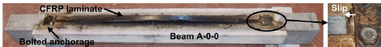
Figure 11. Cable mechanism behavior of the CFRP laminate after fire exposure by Firmo and Correia (2015) [15].
